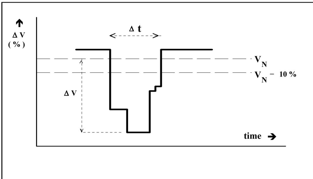
FIG. 2 Simplified form of a voltage dip
