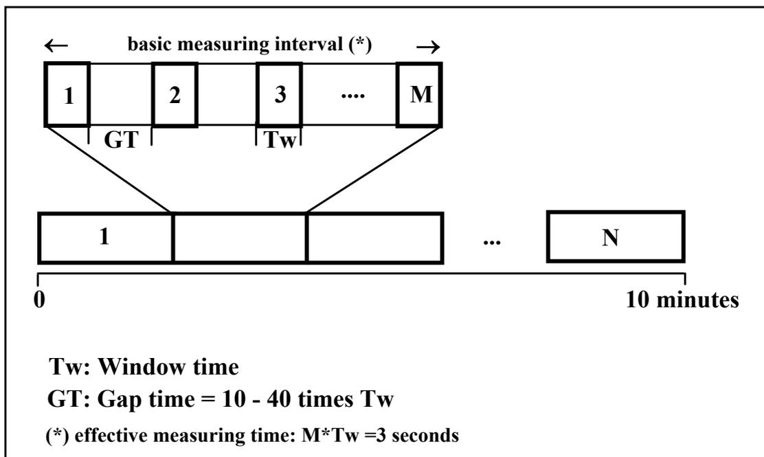
FIG.A1 Scheme of measuring timing for harmonics
