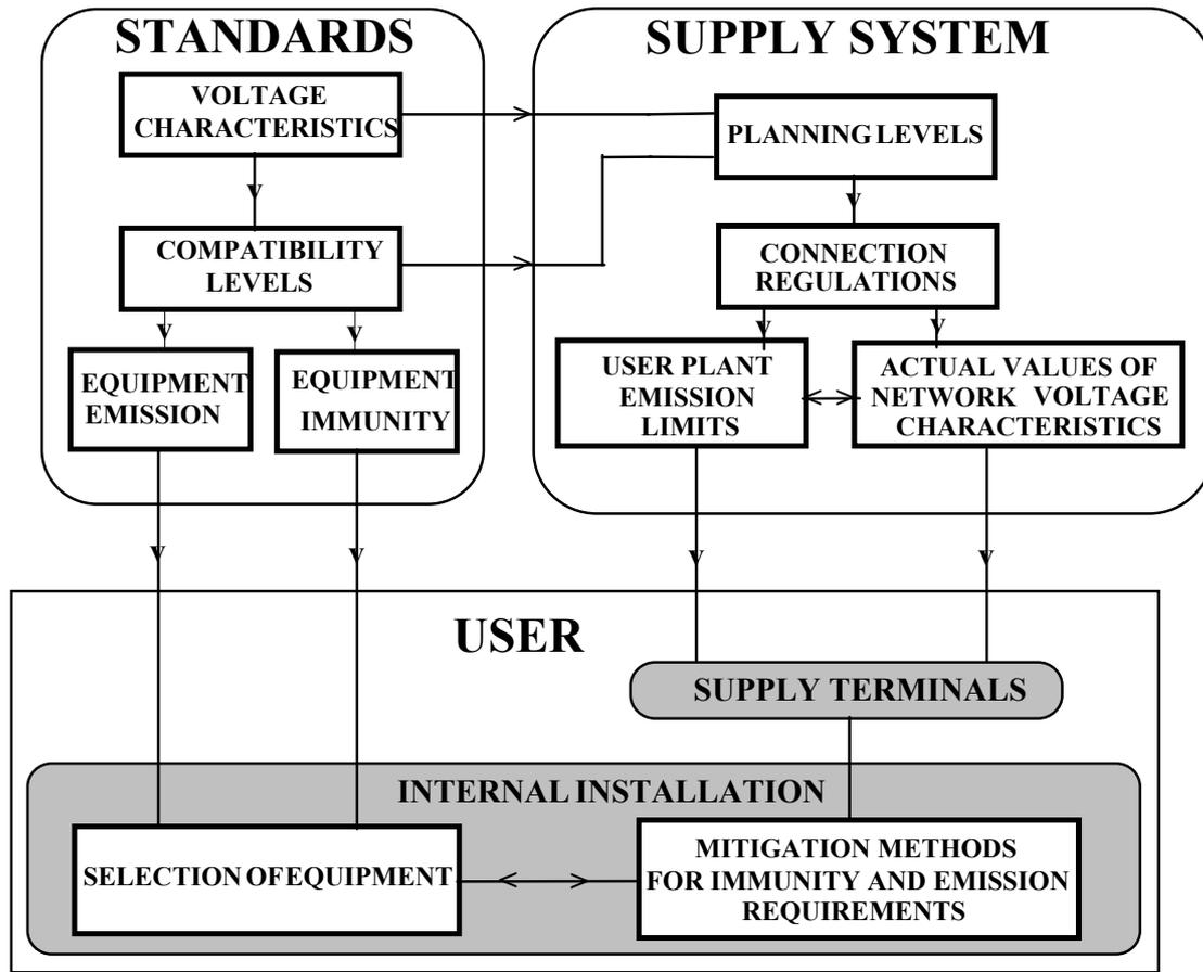
FIG. 5 Relation between standardisation, management of voltage characteristics, user equipment and installation options
