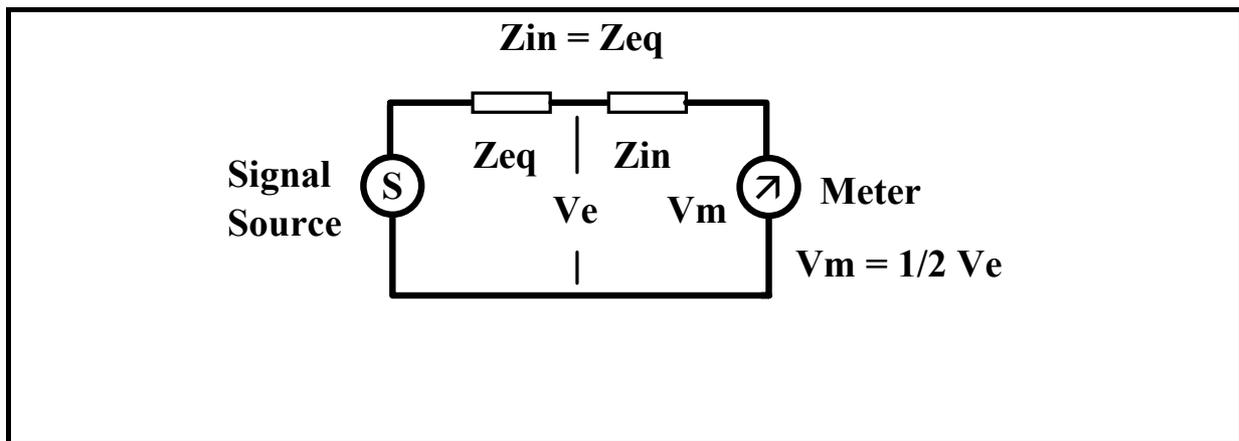
FIG. 3 Measuring arrangement for injected signals
