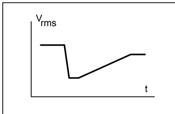
FIG. 1 Schematic form of a rapid voltage change
